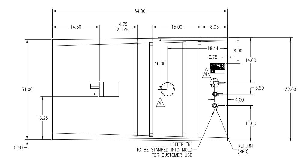
NOTE: DOGHOUSE IS 5.98 LONG, 4.50 WIDE, 2.25 TALL, & HAS A 1.25 TOP FLAT. RIBS ARE 1.00 WIDE, 1.00 TALL, 1.00 FROM EDGE OF TANK, & BEVELED 45.00° AT ENDS.
